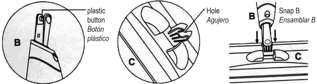
Remove cap from cartridge (E) and click into place on lower mop pole (B).
